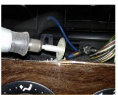
These need to be carefully filed away to allow a Double DIN head unit to fit.
