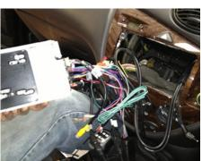
With a 29-606 and a patch lead to suit the make of head unit, connect and test the operation of the steering wheel controls.
