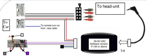
1-ALWAYS CONNECT THE HEAD-UNIT CABLE ADAPTER 1st before ignition is turned on!
