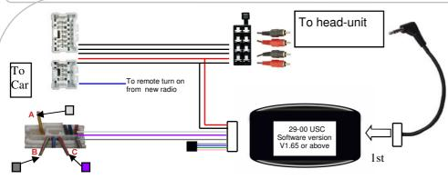
1-ALWAYS CONNECT THE HEAD-UNIT CABLE ADAPTER 1st before ignition is turned on!
