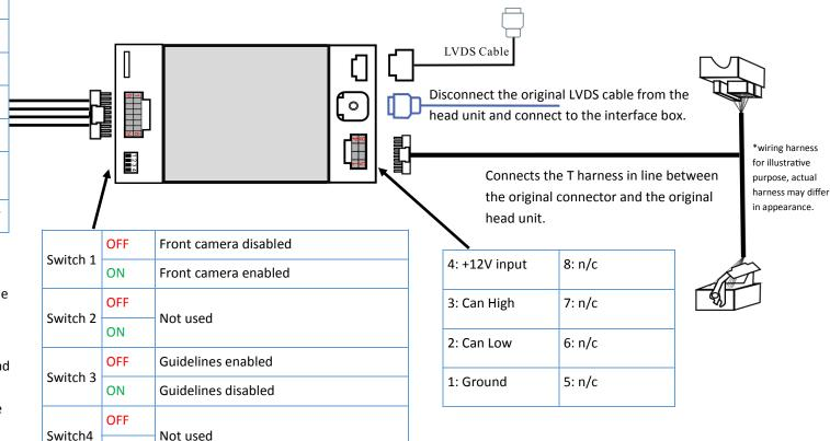
The switches need to be set before the interface is powered. If the switches need to be changed the interface will need to be disconnected from the power to reset.
