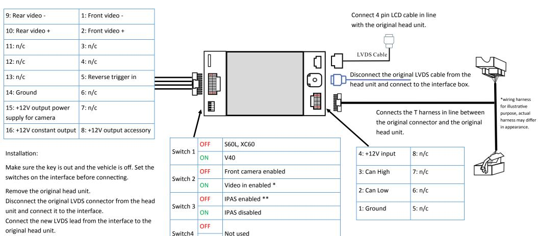
Disconnect the connector at the head unit and fit the supplied T lead in line.
