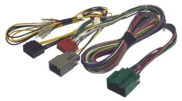
Disconnect the green and grey connectors at the amplifier and connect to the 20-307. Run the 20-307 up through the dashboard to the new head unit. Connect the ISO connectors to the new head unit.
