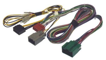
Disconnect the green and grey connectors at the amplifier and connect to the 20-307. Run the 20-307 up through the dashboard to the new head unit. Connect the ISO connectors to the new head unit.
