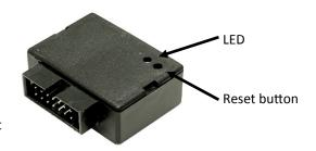
As the interface is prewired for ignition, the first output will need to be confirmed as ignition. Press and hold the reset button for 3-5 seconds, this will confirm the selection.
