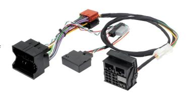
When fitted the interface will automatically recognise the vehicle, the LED on the interface will light up green when the ignition is on. If the LED flashes red this means the interface has not recognised the car, check the CANbus wires are mating, also disconnect and reconnect the interface and cycle the ignition a few times.
