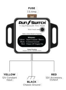
YELLOW: Connect directly to a 12V battery (+) terminal. This is the INPUT power to the RunSwitch module and requires a constant power connection directly from the 12V battery.
